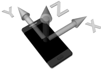
Figure 1: Axes of acceleration
